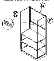
6 Insert (H) Right Header Frame into the tube located at the rear of (C) Right Side Frame. Tighten them with two (K) M6x10 Hex Screws.
