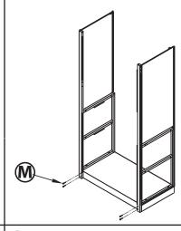
4 Install (D) Middle Shelf first by using four (M) M6x35 Hex Screws threading through the Side Frames and tightening with (AA) Allen Key. Repeat for (E) Top Shelf.
