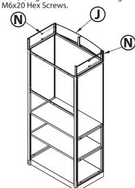
8 Align tab coming off of (B) Left Side Frame with the hole located on the bottom of the (I) Left Header Frame and secure using one (K) M6x10 Hex Screw. **Repeat steps** to secure (H) Right Header Frame to (C) Right Side Frame.
