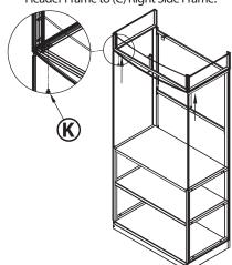
9 Slide (T) Bottom Back panel into bottom rear channels located at the back of Display.
