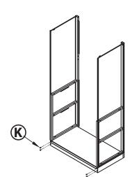
3 Continue to secure (B) Left Side Frame to base using two (M) M6x35 Hex Screws at the holes located on the back of the (A) Base using the (AA) Allen Key. Repeat to secure (C) Right Side Frame.
