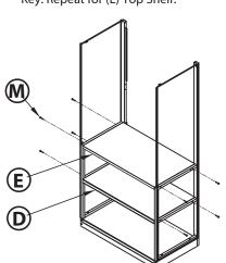
Secure (F) Middle Back Brace to Side Frames using four (K) M6x10 Hex Screws.
