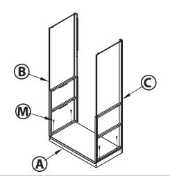
2 Continue to secure (B) Left Side Frame to base using two (K) M6x10 Hex Screws at the holes located on the front of the (A) Base using the (AA) Allen Key. Repeat to secure (C) Right Side Frame.
