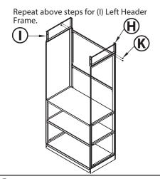
7 Secure (J) Center Header Frame to (I) Left and (H) Right Header Frames using four (N)
