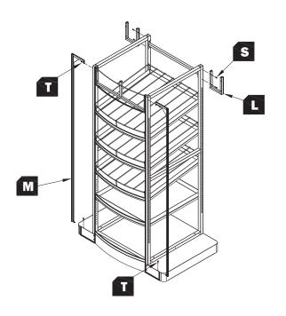
6 -Attach (G) Side Header Frames to (L) Back Header Frame and (M) Front POS Frame with x4 (S) Medium Bolts each and tighten with (U) Tool. -Attach each (E) Side Base Shelf to (B) Side Frame with x3 (T) Short Bolts each and tighten with (U) Tool.
