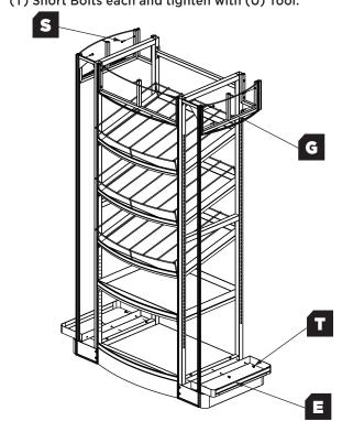
Install (N-Q) Back Header and POS Graphics by sliding into respective channel slides.
