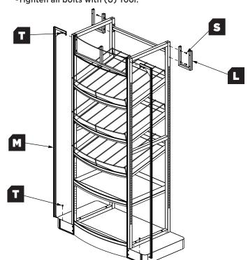
6 -Attach (G) Side Header Frames to (L) Back Header Frame and (M) Front POS Frame with x4 (S) Medium Bolts each and tighten with (U) Tool.
