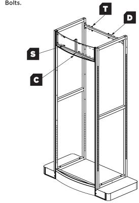
4 -Thread x4 (T) Short Bolts into each (H) Center Angled Shelf location on the (B) Side Frames but leave loose. -Place the (H) Center Angled Shelves onto the protruding (T) Short Bolts, then tighten with (U) Tool.
